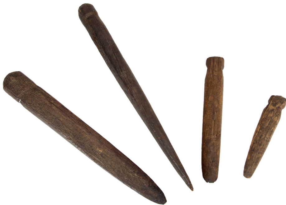
Wedges (kahi) were made of hardwood such as mānuka, and pounded by a wooden mallet (tā) into an adzed surface of a tōtara log to split off a flat slab for building and carving. Auckland War Memorial Museum
